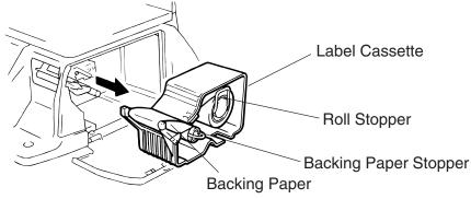
**NOTE:** When removing the backing paper, loosen the paper by turning the paper winding shaft counterclockwise.
